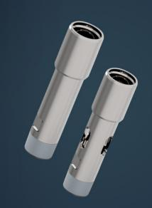
PCM Tag Bar is a specific accessory for PCP completion to land the rotor properly against the stator. The Tag bar is used in any rod driven PCP completions and is connected to the bottom end of the stator. The Tag Bar is a key item in completion for spacing out and shall ensure the maximum PCP inflow.
