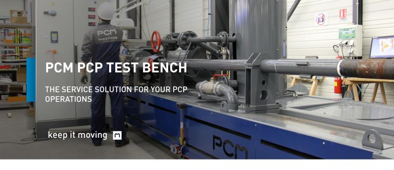
Double check performance of your new PCP before run in hole or requalify some of your used PCP to reduce your CAPEX with PCM PCP service test bench.
