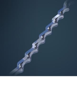
Paddle rotor is equivalent to standard rotor coming with 2 feet extra length chromed rotor and flat surface machined. The Paddle part is running at PCP suction and allows to break solids accumulation before it goes through the stator.
